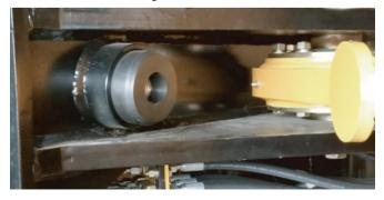
The steering limit is pre-limited by rubber, which makes the limit more stable.
