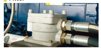
The transmission adopts a new type of high-precision and large-flow Filter, which is easy to remove and replace the Filter element and more convenient for maintenance.
