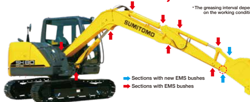
A Solid lubricant B Dust seal Plated pin High strength brass Special bushing A A solid lubricant embedded in high strength brass forms a layer on the bushing surface to prevent contact between metals, maintaining an excellent lubricated state to reduce abrasion of joints. B The surface of the pin is plated to increase surface hardness and improve wear resistance.
